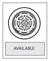
If your pin connector matches the image, your vehicle supports the standard 7-pinround connector
