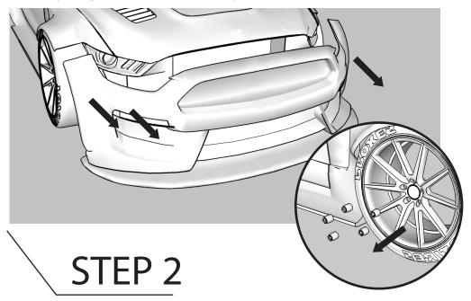
Unplug the two plugs from the stock turn signal and the one from the fog light
