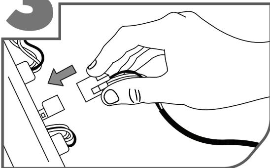
Connect the electrical plug to your new brake light housing.
