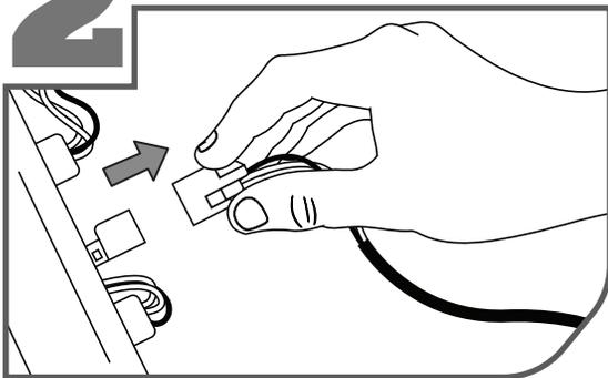
Disconnect the electrical plug from the original brake light housing.
