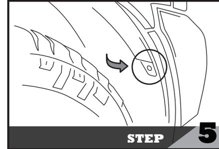
Remove the 10mm bolt (1x) to open the fender liner.
