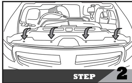
Remove the 10mm bolts(4x) from the grille as shown in step 2.
