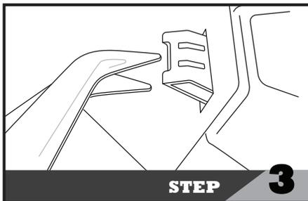
Remove the front grille by releasing (6x) retaining clips.
