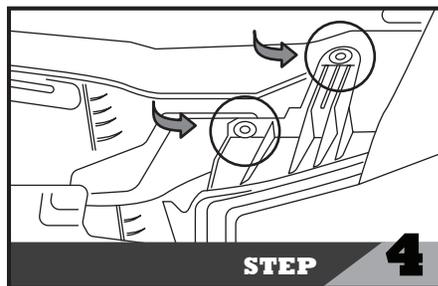
Remove the 10mm bolts (2x) from the OEM headlight as shown in step 4.
