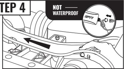
Run the wires along the front brace and connect to the control box.
