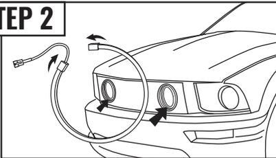
Wrap the LED strip into a circle shape and firmly press into place inside of the intake hole to secure.
