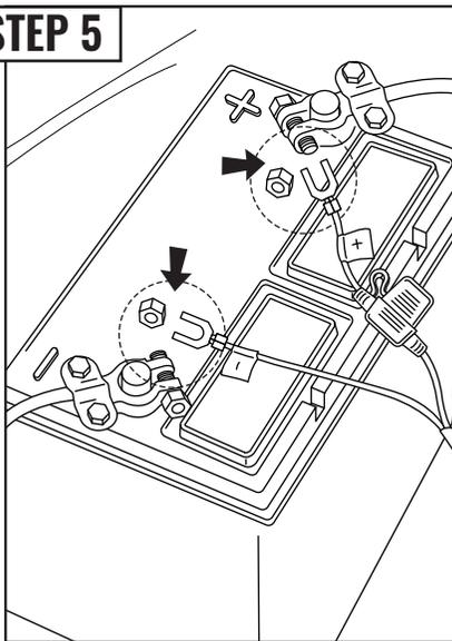
Connect the power wire harness to your vehicle battery.
