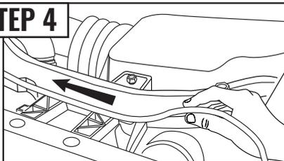
Run the wires along the front brace and connect to the control box.
