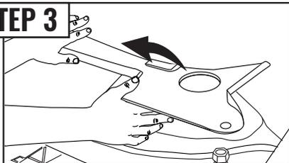
Remove the plastic covers on the right and left side of the engine bay.
