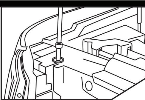
Remove the 2 bolts on top of the headlight.
