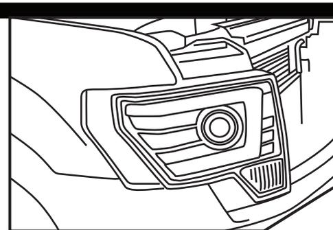
Line up the headlight housing mounting tabs and push rearward to seat it in place.
