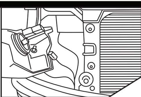
Reattach the electrical connectors to the new headlight housing.
