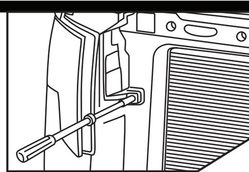
Remove the last bolt retaining the headlight.
