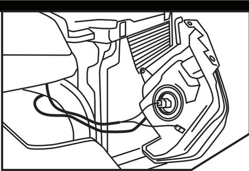
Unclip the electrical connectors on the back of the headlight housing.
