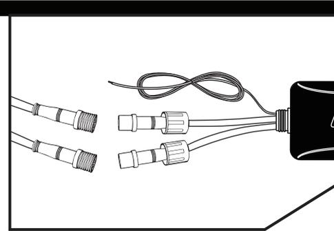
Connect the round connector from the headlight housings to the control box.
