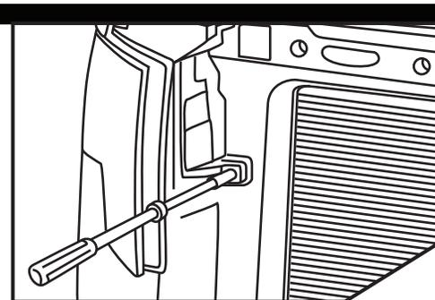
Attach the 3 bolts to secure the headlight in place
